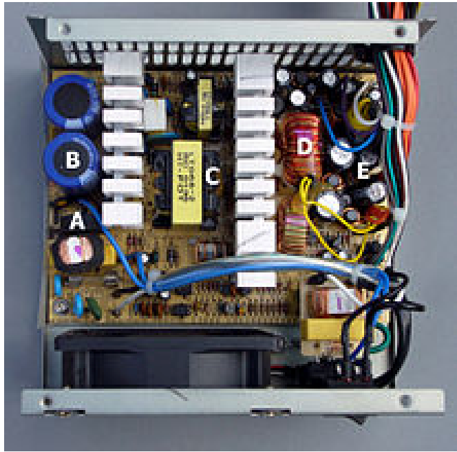
ATX power supply interior
